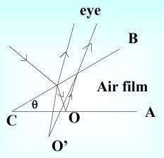
The interfering rays do not enter the eye parallel to each other but they appear to diverge from a point near the film.
