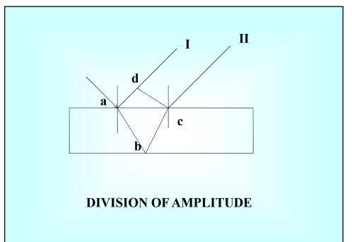
If plane wave falls on a thin film then the wave reflected from the upper surface interferes with the wave reflected from the lower surface.
